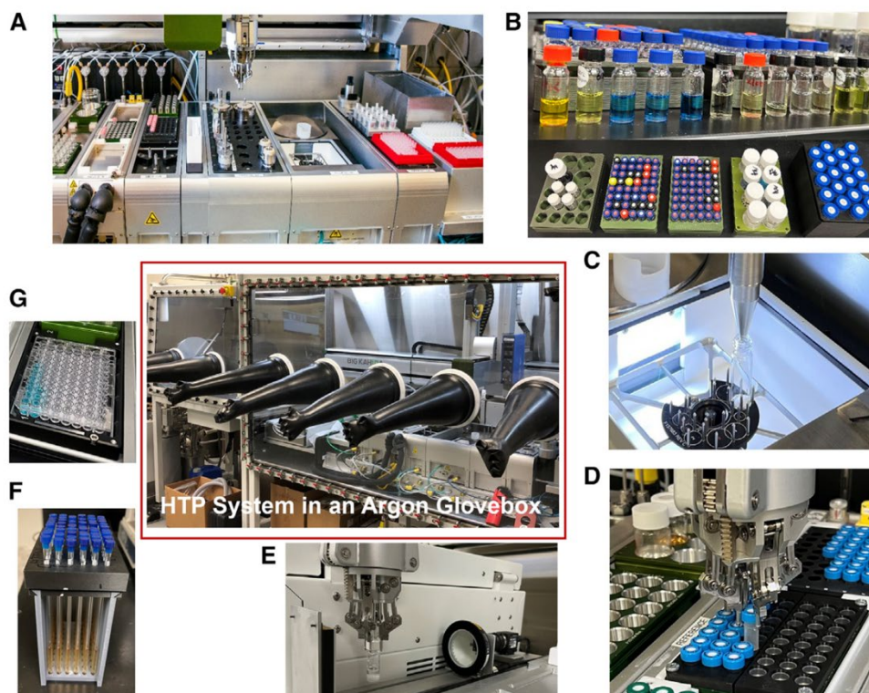
Figure 11. Photographs of a customized robotic platform (Big Kahuna, Unchained Labs) with key functions listed (A) Inside view of the platform. (B) Sample vials and plates used on the platform. (C) Solid/powder dispensing in a balance chamber. (D) Press-filtration plate. (E) On-deck high-resolution camera. (F) On-deck nuclear magnetic resonance (NMR) sample tube holder. (G) 96-well microplate Reprinted with permission from Ref. [25]. Copyright 2023 Cell Reports Physical Science
