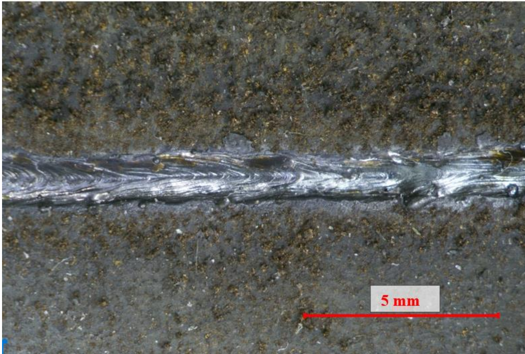
Figure 19. Welded sample with conventionally cleaned side as a pre-treatment.
