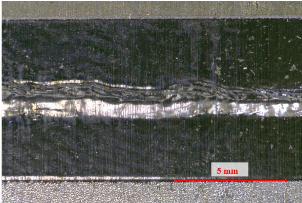
Figure 29. A microscope image of laser cleaned and laser polished sample. Red line indicates scale, which is 5 mm.
