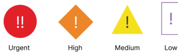
Figure 5.2: Rockwell guideline on hierarchy of alarms (adapted from [38])
