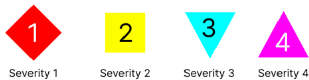
Figure 5.3: AVEVA guideline on hierarchy of alarms (adapted from [39])
