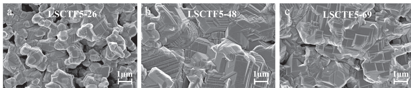
Figure 2. SEM images of porous (a) \text{La}_{0.21}\text{Sr}_{0.48}\text{Ca}_{0.26}\text{Ti}_{0.95}\text{Fe}_{0.05}\text{O}_{3-\delta} (LSCTF5-26), (b) \text{La}_{0.21}\text{Sr}_{0.26}\text{Ca}_{0.48}\text{Ti}_{0.95}\text{Fe}_{0.05}\text{O}_{3-\delta} (LSCTF5-48) and (c) \text{La}_{0.21}\text{Sr}_{0.05}\text{Ca}_{0.69}\text{Ti}_{0.95}\text{Fe}_{0.05}\text{O}_{3-\delta} (LSCTF5-69) electrodes after 5 h sintering in air at 1250 °C.
