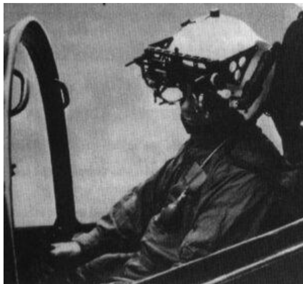
Figure 5: The VITAL helmet, designed by the McDonnell Douglas Corporation. [23]
