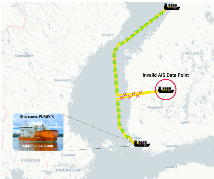
Figure 4. An invalid ship trajectory in the Baltic Sea.
