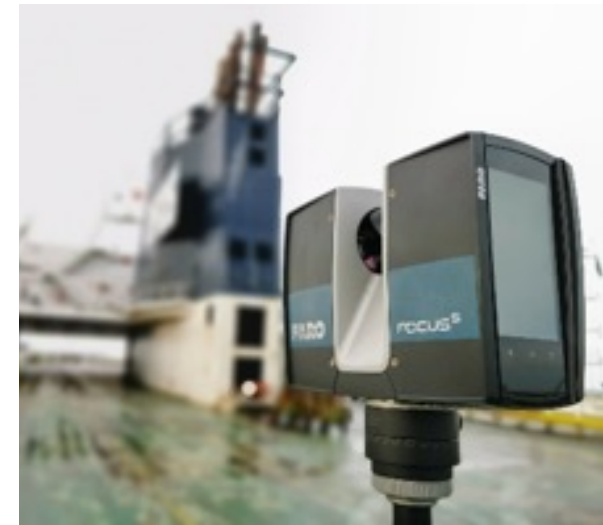
Equipment for 3D Scanning applied on a DFDS vessel to scan Cargo Decks.(Gothenburg Port, September 2021)
