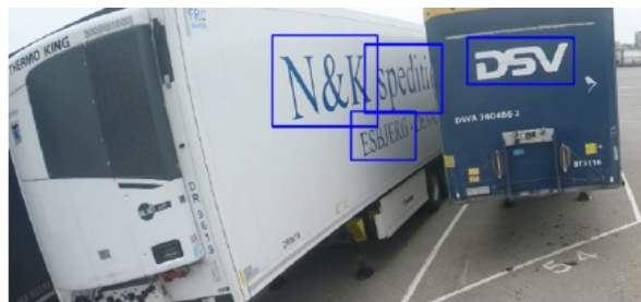
Example on testing/evaluation of two alternative Machine Learning Algorithm detecting trailer logo and trailer IDs. (Esbjerg Port, March 2021)
