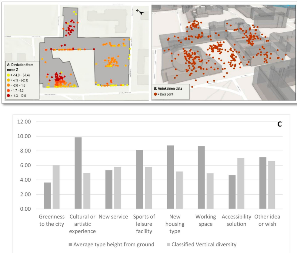
Figure 6. Application of 3D PPGIS metrics in Aninkainen study area: (A) Vertical diversity expressed as the deviation of mean Z for points within the building, (B) An overview of markings within the block area, and (C) Average heights per marking type and classified vertical diversity
