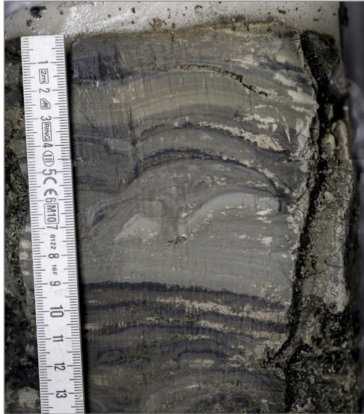
Figure 9. The topmost 13 cm of the varved sediment of Maljalahti Bay, MAL1. The photograph was taken of the fresh freeze core sample.
