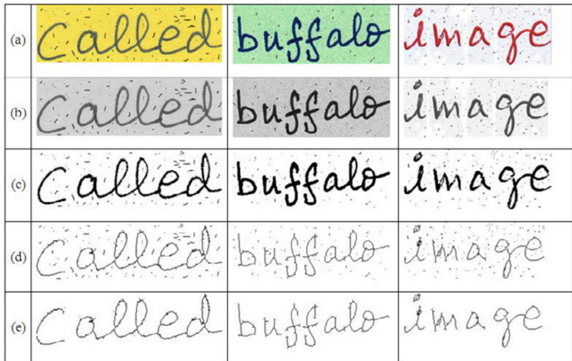
Figure 2.9: An example of pre-processing. (a) input image; (b) translation to grayscale; (c) binarization; (d) thinning; (e) noise removal [41]
