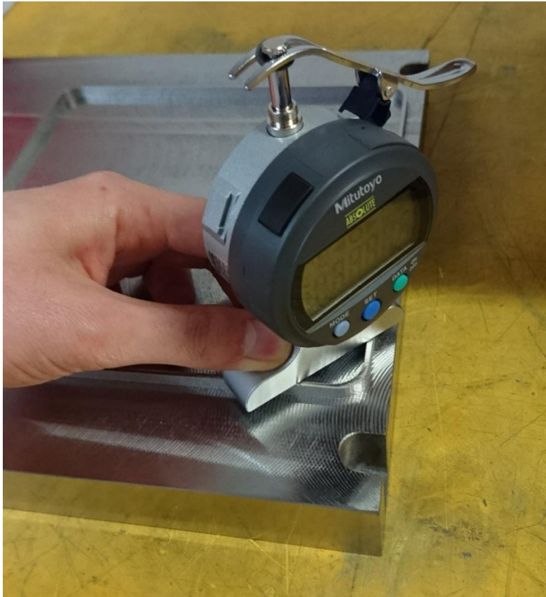
Figure 36 Wall height measurement method with digital depth gage.
