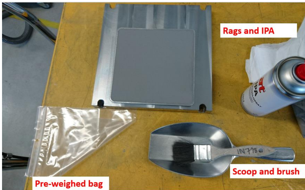
Figure 31 Equipment used for removing sampled powder.
