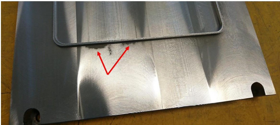
Figure 35 Residual powder outside sampling area, marked with arrows.
