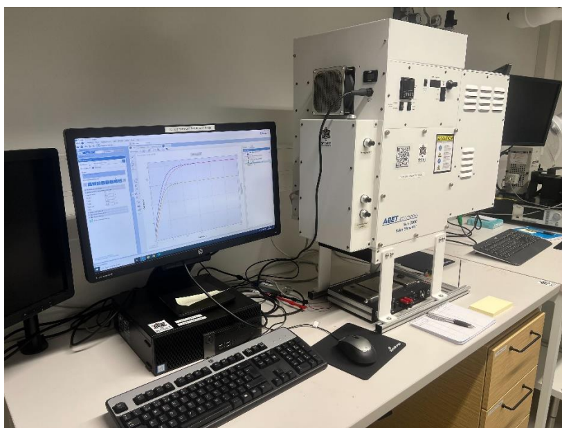
Figure 16. Setup of the Abet 10500 solar simulator utilized for PV characterization.
