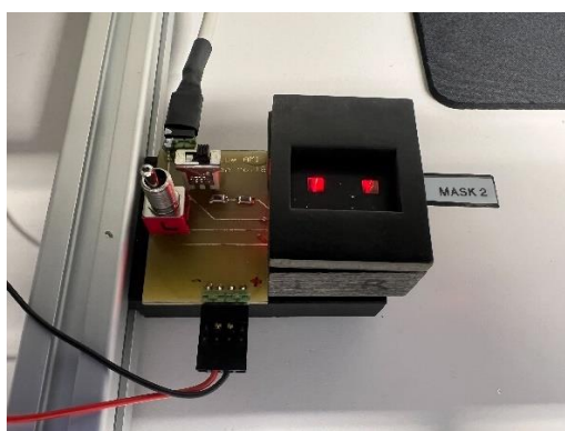
Figure 17. A sample holder with a mask used in I-V measurements of 2-pixel devices under Abet 10500 solar simulator. The exposed windows are marked by the red glowing areas, places where the light from the lamp is directed onto the active area of the solar cell. Regarding the connectors, the red and black wires maintain the connection to the positive and negative terminals of the solar cell, respectively, feeding the current to or from a source-measure unit during measurements. The 'L' label corresponds to the 'left' pixel of a 2-pixel device and indicates a particular test channel.
