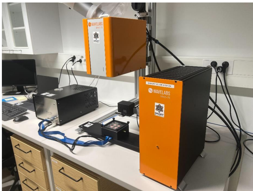
Figure 19. Setup integrating the Wavelabs Sinus 70 solar simulator with the Fluxim Litos Lite measurement platform.
