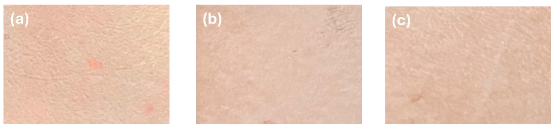
Figure 24: Colour change over time for CuNW-160-PC films (a) 0 hours (b) 14 days (c) 60 days.
