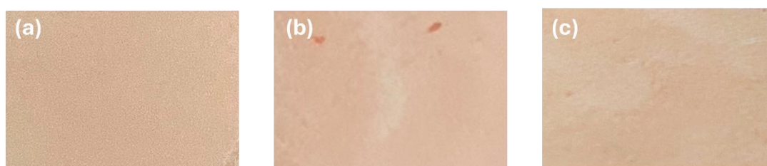
Figure 23: Colour change over time for CuNW-140-PC films (a) 0 hours (b) 14 days (c) 60 days.
