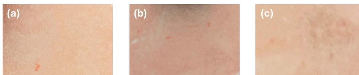
Figure 25: Colour change over time for CuNW-180-PC films (a) 0 hours (b) 14 days (c) 60 days.
