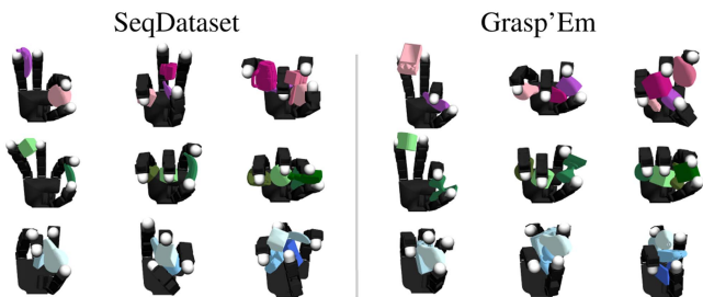
Fig. 5. Qualitative results. For SeqGrasp (first row) and SeqDiffuser (second row), the grasp sequences are visually indicated by a color gradient, transitioning from lighter to darker shades. In contrast, for MultiGrasp (third row), the color gradient is only used to differentiate the objects. For SeqGrasp and SeqDiffuser, we only show consumed grasps, that is, when \mathcal{O}_S = \emptyset .
