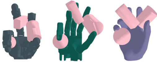
Fig. 2. Multi-object grasping visualizations for different hands. From left to right: Allegro Hand, Shadowhand, MANO.
