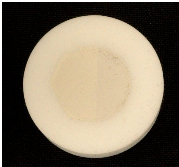
Figure 6. Right side of \text{Na}_8\text{Al}_6\text{Si}_6\text{O}_{24}(\text{Cl}_{10\%}, \text{S}_{75\%})_2 sample irradiated with 254 nm for 5 min, left side covered during irradiation. The photo has been enhanced to properly display the colour change.
