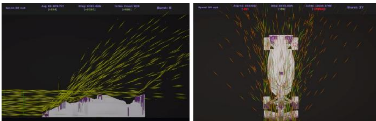
Figure 9. CFD simulation of a voxel-based Formula 1 car [25]. © 2024 IEEE
