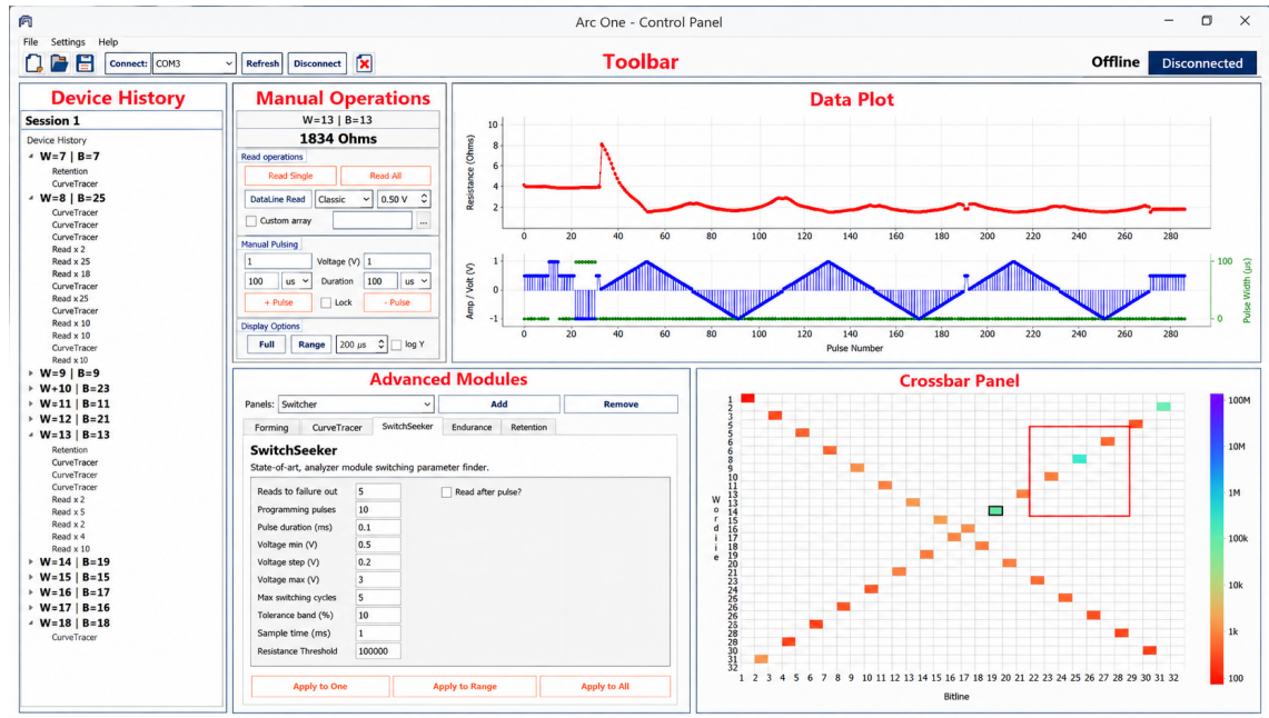
Figure 19. Device History, Manual Operations, Toolbar, Data Plot, Advanced Modules, and Crossbar Panel are the functional panels of the Arc ONE user interface [93].
