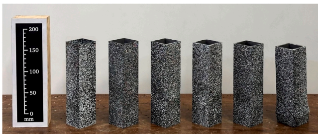
Fig. 18. Deformed PBF-LB/M SHS stub columns, with increasing wall thickness from left to right.
