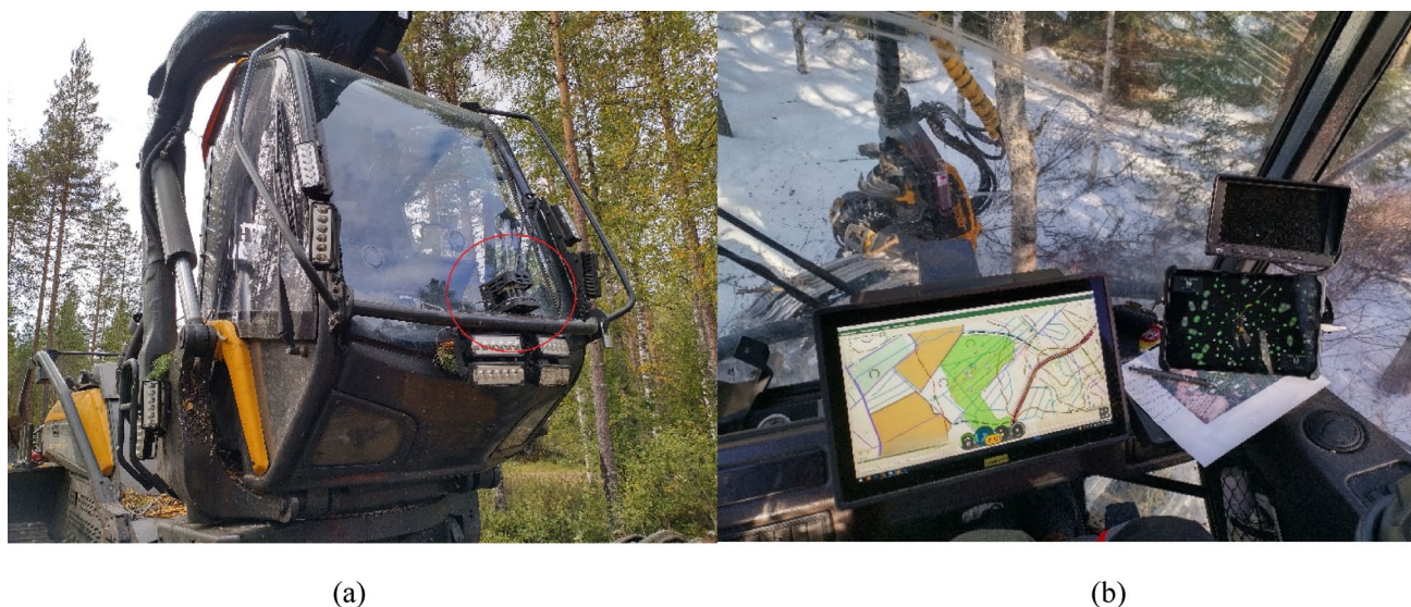
Fig. 2 a The Ouster LiDAR OS0 (indicated by a red circle) on the cabin front of the Ponsse Scorpion King, and b the view from the harvester cabin
