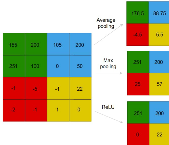
Figure 4: Operation of the Average Pooling layer, Max pooling and Rectified Linear Unit (ReLU) to reduce the dimensionality.
