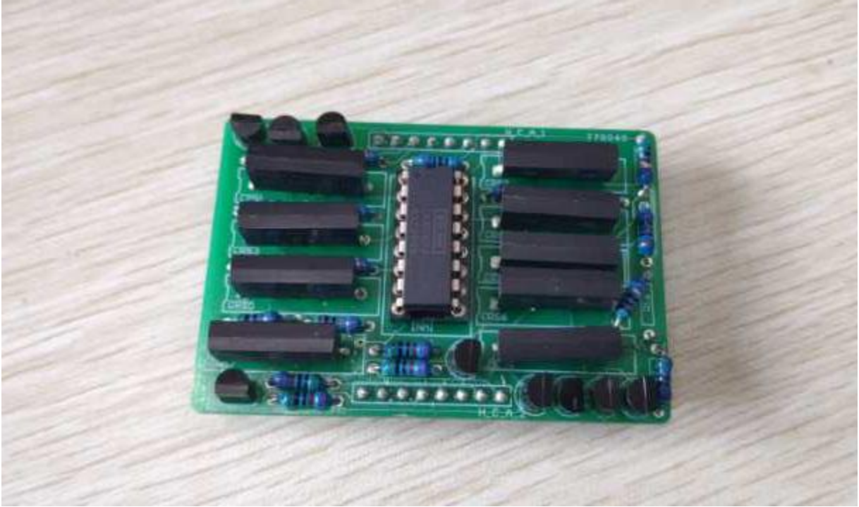
Figure 9: Final work of high-side current amplifier
