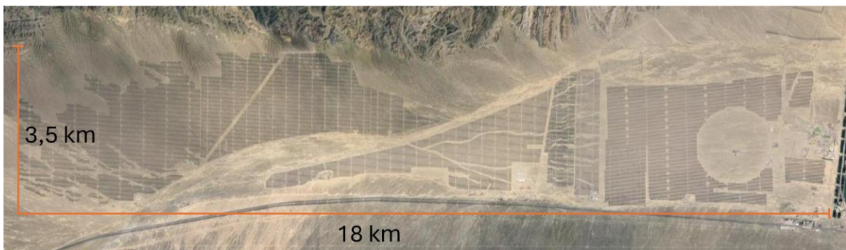
Figure 5 Satellite image from Xinjiang solar farm, the largest operating solar farm in the world. The panels are spread in a 18 km × 3.5 km area in the desert area. Image modified from Google Maps [44].
