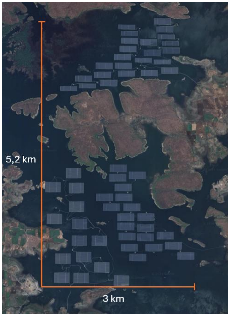
Figure 7 Satellite image from Kwanda solar park, the largest operating floating solar park in the world. The panels are spread in a 5.2 km × 3 km area in the Omkareshwar dam area. Image modified from Google Maps [44].
