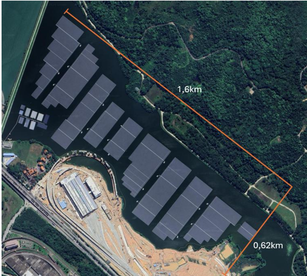
Figure 8 Satellite image from Sembcorp floating solar farm, Singapore. The panels are spread in a 1.6 km × 0.63 km area located inside Singapore water-area. Image modified from Google Maps [44].
