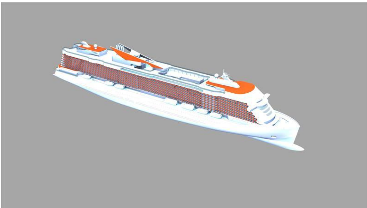
Figure 9 Illustrated picture of AVATAR110 concept ship. The reserved PV panel installation area is painted orange in the ship. In total, there are 5428 m 2 worth of installation area for PV panels on AVATAR110. Image courtesy of Meyer Turku.
