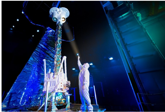
Fig. 3 Photograph of IXPE with the boom deployed in a TVAC during Observatory environmental testing. When deployed, IXPE is 5.2 m from the bottom of the spacecraft structure to the top of the payload and is 1.1 m in diameter. The solar panels, removed for TVAC, span 2.7 m when deployed. Photo courtesy of Ball Aerospace.
