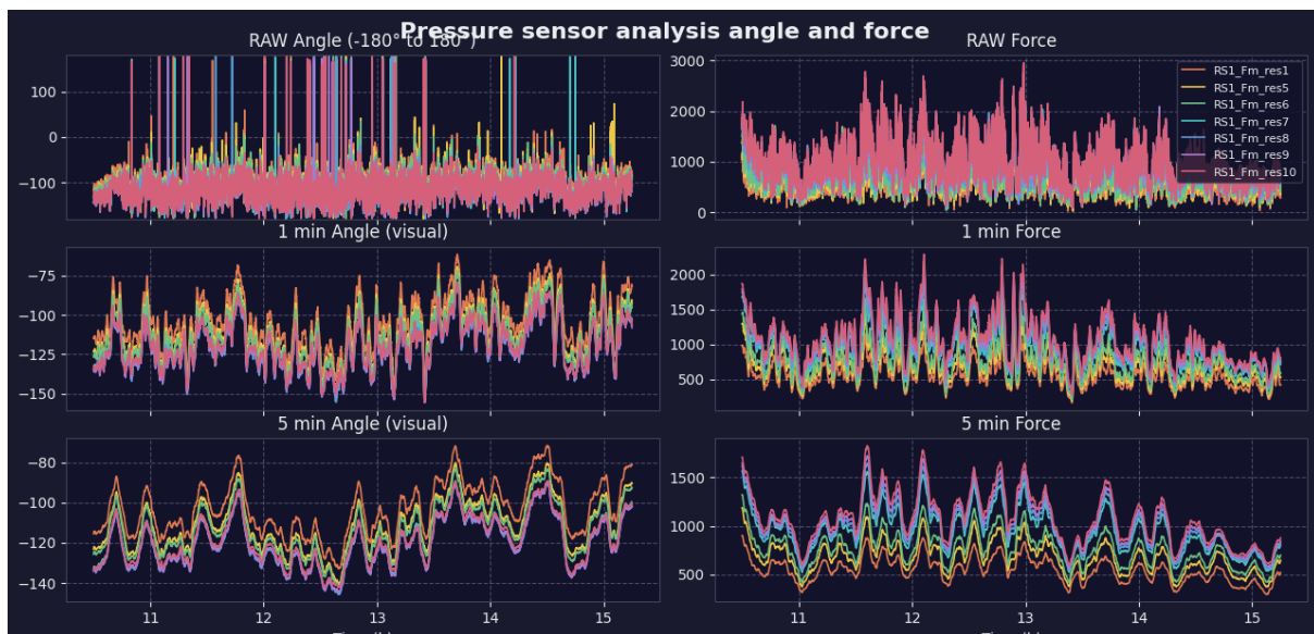
Figure 21: Force calculation plot, MAG and DIR, rolling avg
