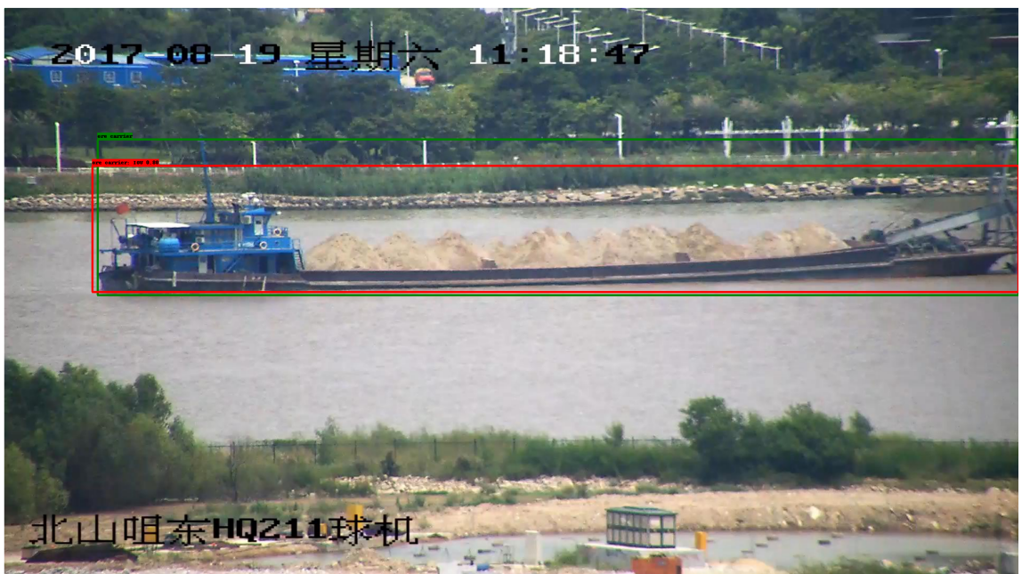
Figure 3.1: IoU (0.80) of a vessel detection, image from SeaShips and overlays by the author – ground truth bounding box in green, predicted bounding box in red.
