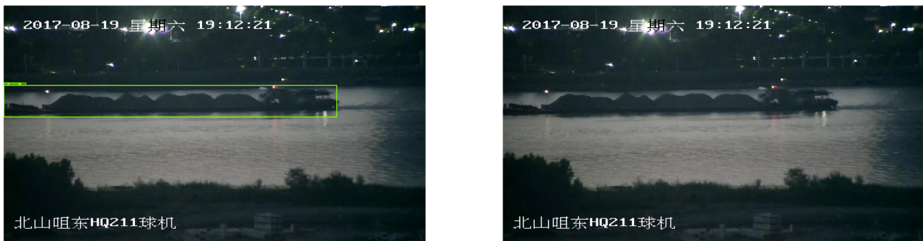
Figure 5.5: A late evening image from SeaShips test set, with detection score threshold of 0.3. Left: Faster RCNN ResNet 152 with a detection (score \approx 1.0 ). Right: SSD FPN ResNet 152 without a detection (score \approx 0.2 ).
