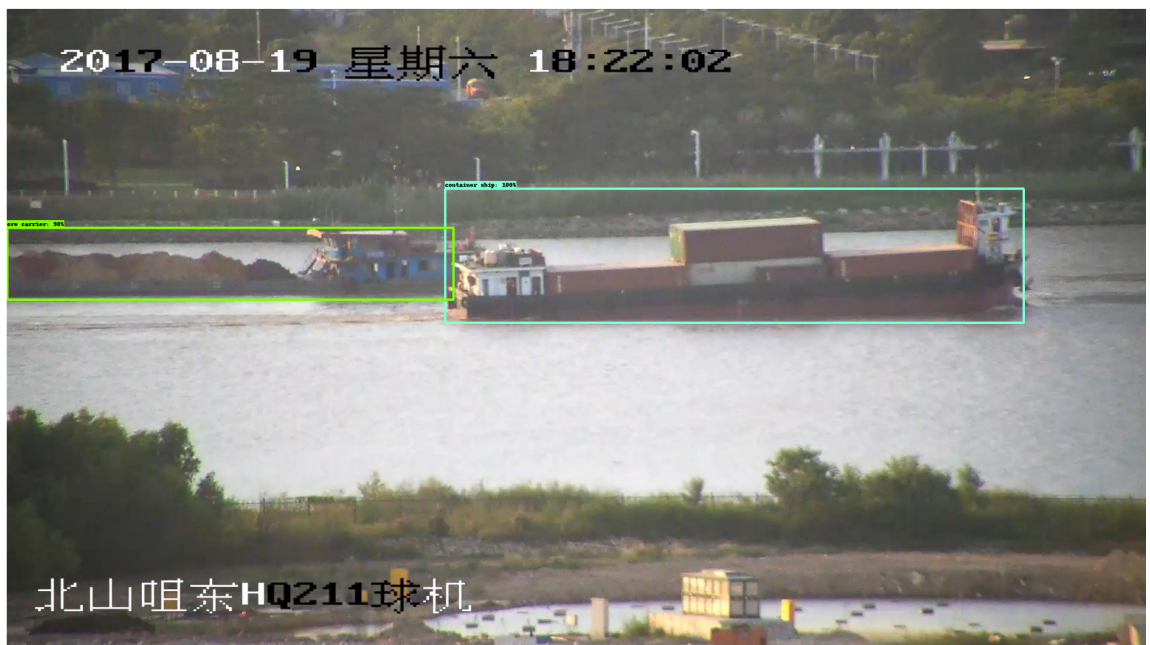
Figure 5.2: Vessel detection example from SeaShips test set using SSD FPN with ResNet 101 backbone.
