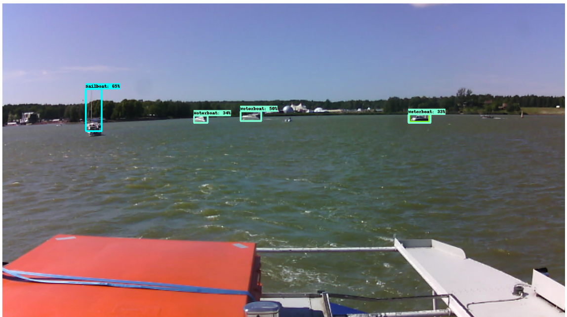
Figure 5.1: Vessel detection example from ABOships test set using SSD FPN with ResNet 101 backbone.
