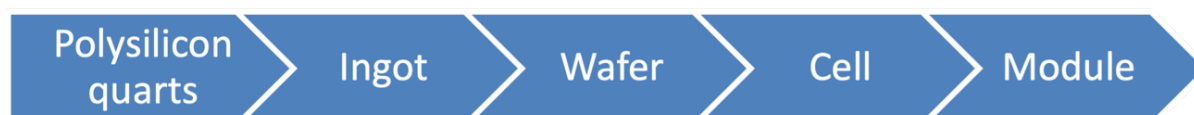
Figure 2. The manufacturing process of a silicon-based solar panel, from quarts to module (U. S. Department of Energy, n.d.).
