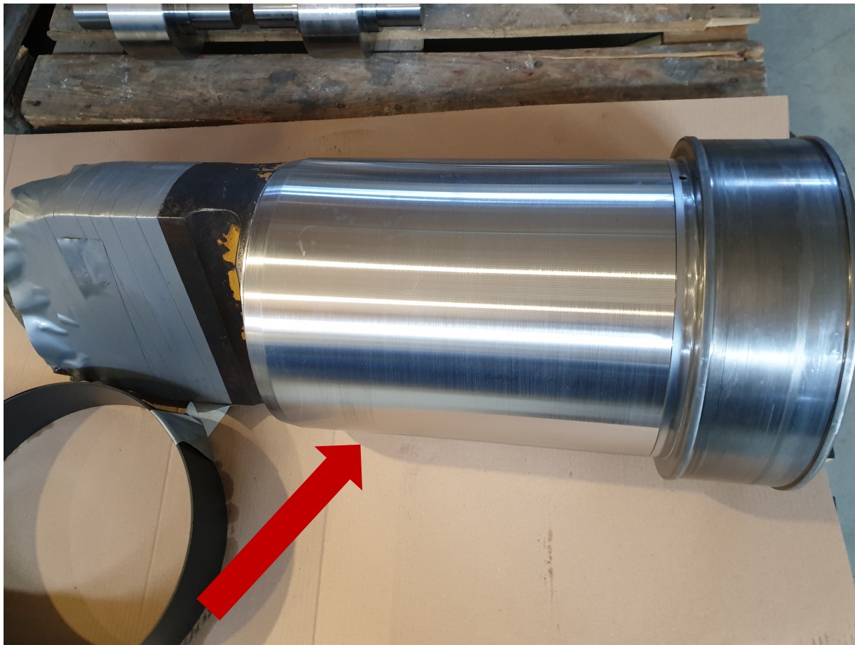
Figure 2. A repaired hydraulic cylinder rod restored using DED-LB. The image shows a similar component type to the one analyzed in this case study (red arrow points to the part that has been worked on).
