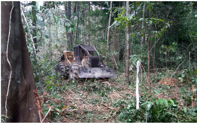
Photo 1. A Skidder is mowing down saplings and poles to do a skid trail for dragging logs to the landing. Fazenda Rio Capim. Paragominas, Pará. 11.12.2021 by Johan Slätis.
