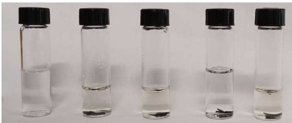
Figure 6. Testing setup for removal of pharmaceuticals from water. The film is placed at the bottom of the vial, and a pharmaceutical solution is added on top of the film. Vials are capped to prevent water evaporation.
