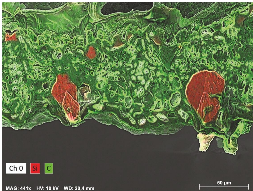
Figure 2. SEM-EDS micrograph of a leaf where phytoliths (red) are located in the upper side of the leaf. The distance between phytolith particles is 120 \mu\text{m} . Original magnification 441 x, bar = 50 \mu\text{m} )
