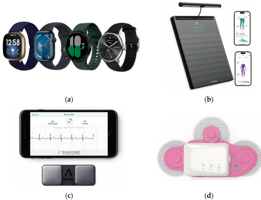
Figure 2.8: ECG wearables: (a) from left to right, FitBit Sense, Apple watch series 4, Samsung Galaxy Watch 4 and Withings ScanWatch; (b) the Withings body scan is a smart scale that displays ECG data acquired via a multi-electrode grip (6-lead); (c) small, portable, medical-grade personal ECG device from AliveCor; (d) ECG patch for continuous monitoring. [17]
