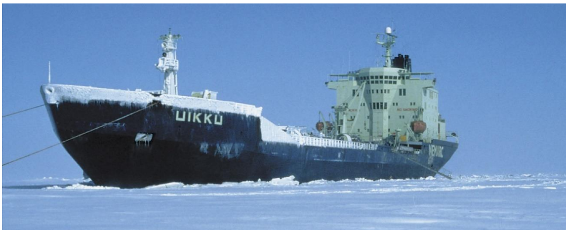
Figure 44. IA Super ice class product tanker with icebreaking bow.
