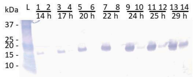
Fig. 9. Time course analysis of Nb3K leakage into medium by western blotting. Resuspended cell pellet samples (odd numbers) and medium samples (even numbers) were probed with HRP-conjugated anti-Histag antibody and precipitating TMB. Pellet samples were diluted 1/5 in H 2 O before loading. L = Protein standard. Sampling time points are indicated under the lane numbers rounded to the closest full hour.
