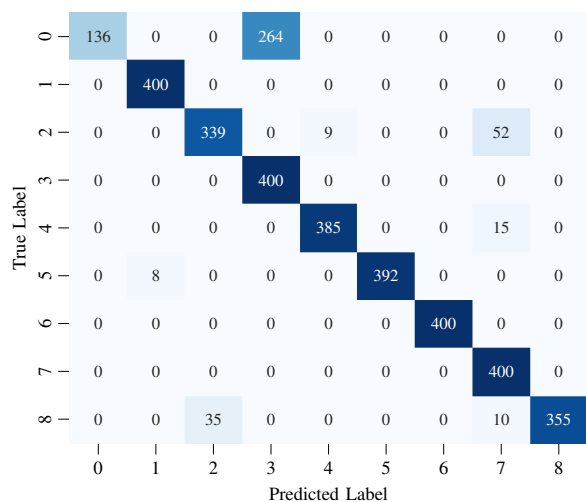
Fig. 5. SVM confusion matrix obtained with leave-one-out cross-validation (iterating over all subjects).
