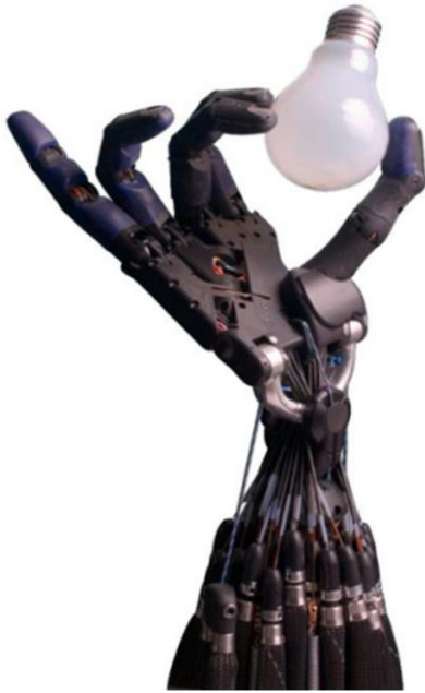
Figure 4: Shadow Hand with pneumatic artificial muscles. Reproduced from [3], used under CC BY 4.0 .
