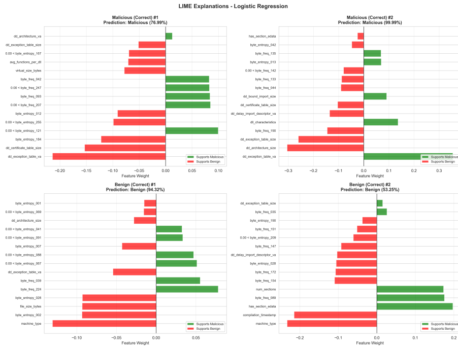
Figure 5.9: LIME explanation for Logistic Regression. The linear model relies more heavily on byte frequency and entropy statistics compared to tree-based models
