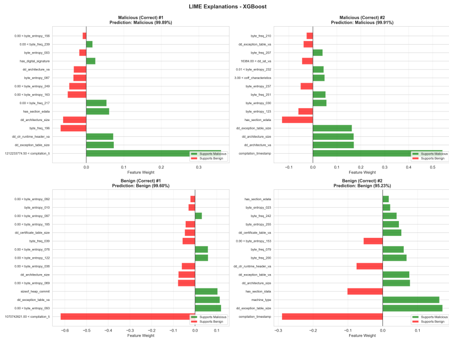
Figure 5.11: LIME explanation for XGBoost on the same malicious sample, showing the top influential features with their importance scores
