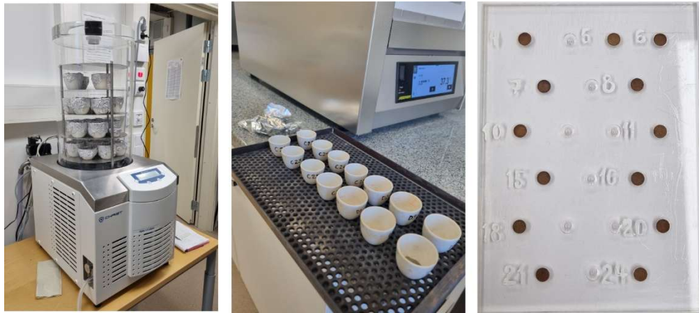
Figure 3. Sample preparation. Samples in the freeze-dryer (left), subsamples after loss on ignition (middle), and basin subsamples on the sample plate prior to \mu -XRF analysis (right).
