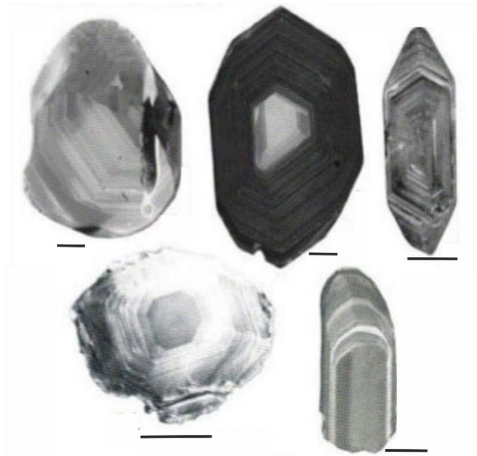
Figure 6. CL images showing magmatic growth zoning patterns in zircons from typical crustal rocks. Relatively simple and fine bands with alternating bright and dark luminescence. Scale bars approximately 50 \mu\text{m} . Modified after Corfu et al. (2003).
