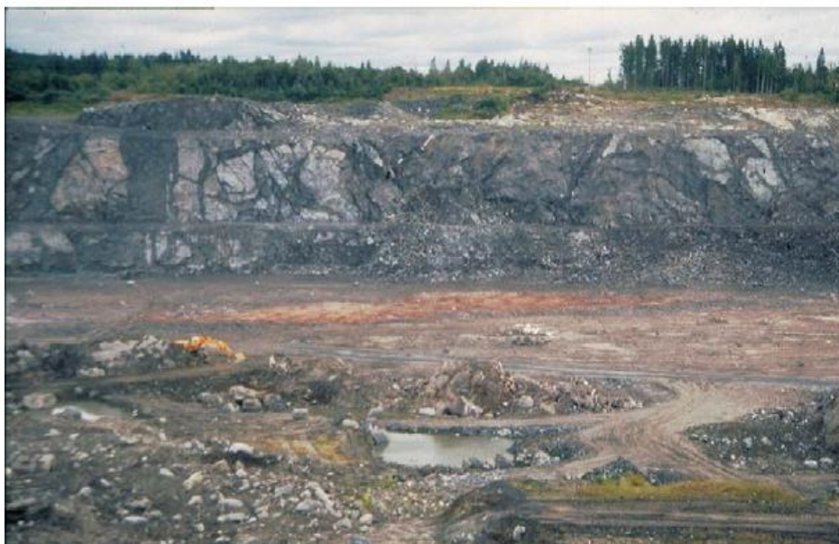
Figure 12. Light fenite blocks in the glimmerite from Siilinjärvi mine. Modified after Lukkarinen (2008).
