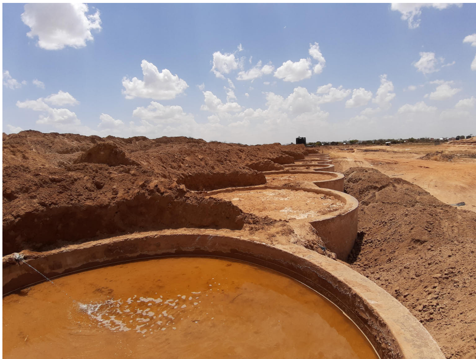
Figure 5. Gold extraction through cyanide. Accumulated mine tailings surrounding the VAT leaching tanks in a gold plant in Kahama District, 2023. Author's photo.
