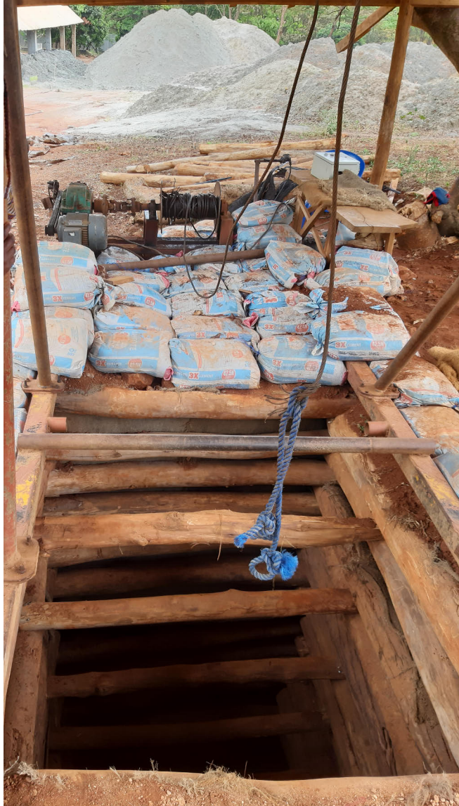
Figure 3. ASGM shaft in Geita featuring a generator-powered electric winch used for hoisting miners and ore. Behind the shaft are bags of ore and sizeable piles of tailings. Author's photo.
