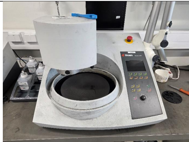
Struers Tegramin- 30 grinding and polishing machine
