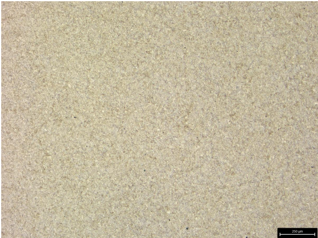
Figure 33 Microstructure of X40CrSiMo 10-2 sample 2 etched with Vilella on 50x magnification.
