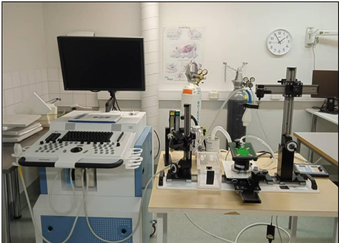
Figure 3: Image of the micro-ultrasound device and its accessory components including the induction chamber, temperature-controlled board, mechanical arm, and movable stage.
