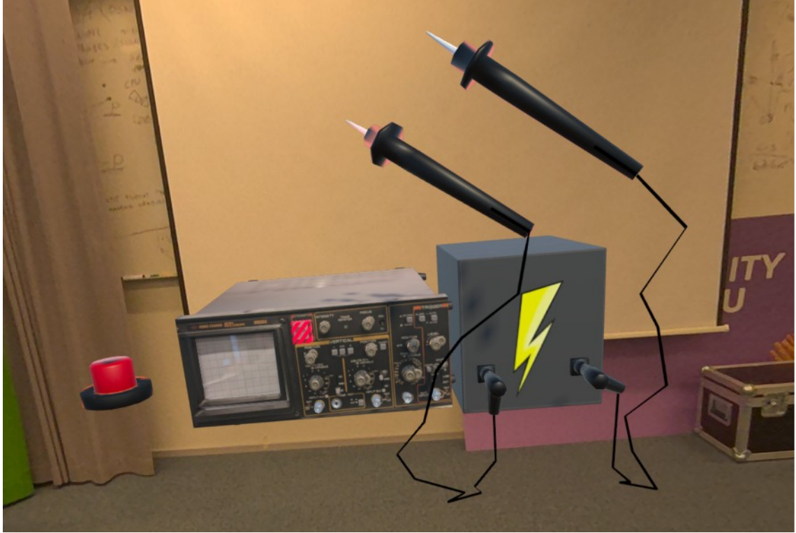
Figure 5.3: The digital model of a oscilloscope within the finalized solution. Included are a mock signal generator and oscilloscope probes.
