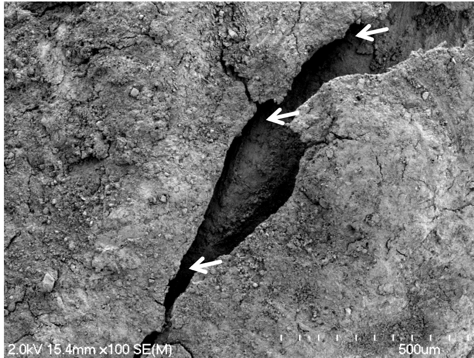
Figure 2: Scanning electron microscope images of the crown/cement interface. White arrows indicate cement explosion, ablation, and hydrodynamic ejection.
