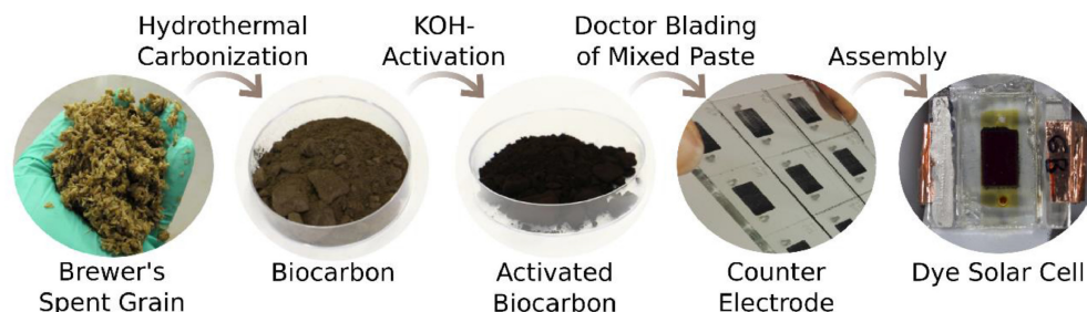
FIGURE 4 Process from brewery residues to dye solar cells with activated biocarbon counter electrodes. Source: Reprinted with permission (Tiihonen et al., 2021).
