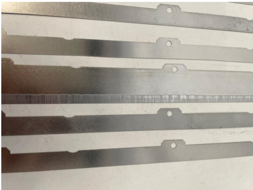
Figure 6. Cold-welded aluminium formed on the wider scraper plate on the inner side of the rotary feeder assembly after eleven building processes.
