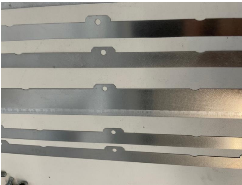
Figure 7. Cold-welded aluminium formed on the wider scraper plate on the inner side of the rotary feeder assembly after first building process.
