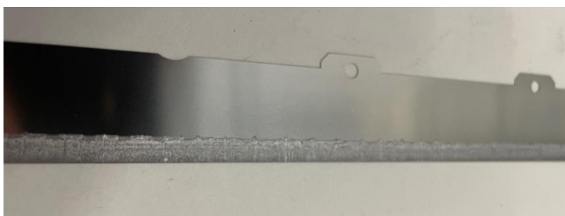
Figure 1. AlSi10Mg adhered on the wider scrape plate of EOS M 400 rotary feeder assembly.
