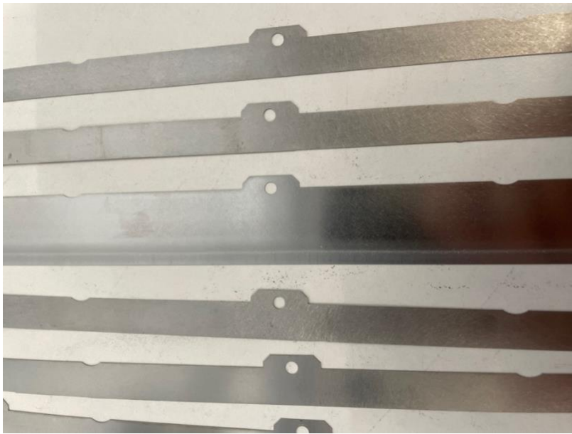
Figure 5. Cold-welded aluminium formed on the wider scraper plate on the outer side of the rotary feeder assembly after eleven building processes.
