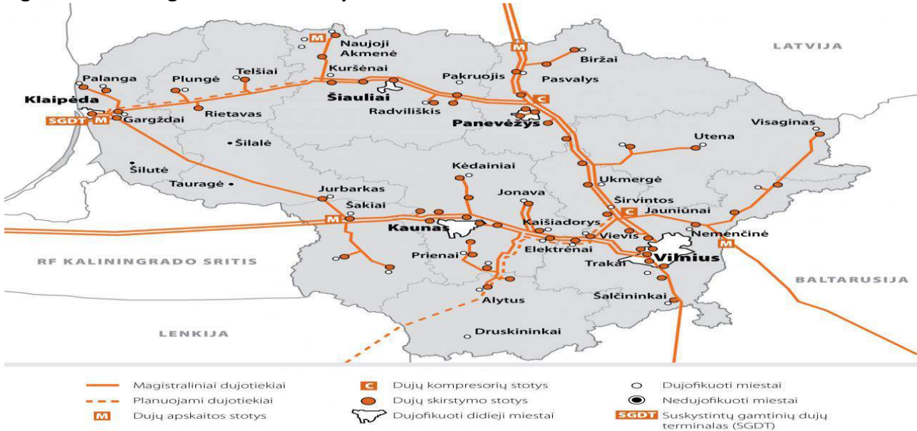
Figure 4. Natural gas transmission system
