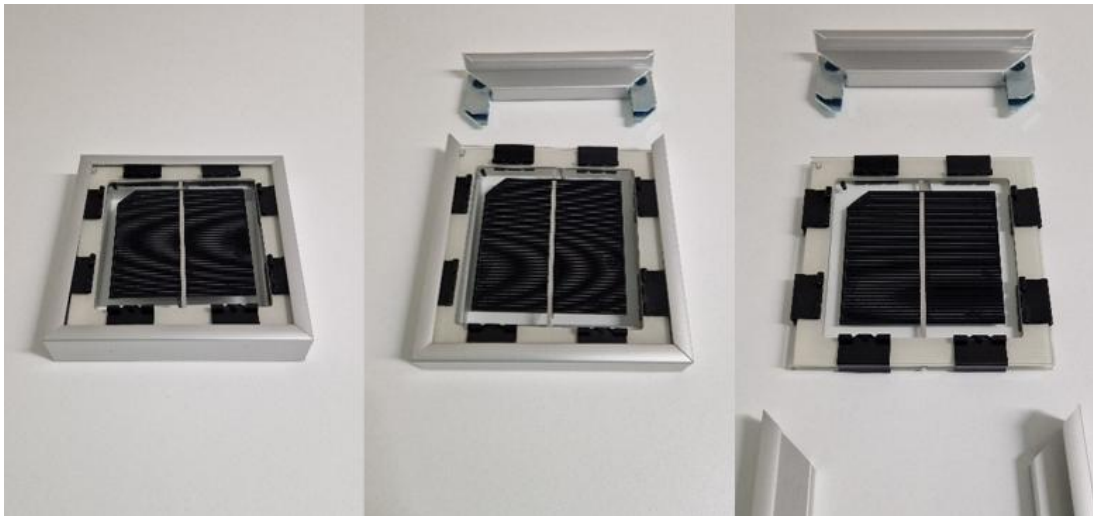
Figure 32. Disassembly of the protective frame
