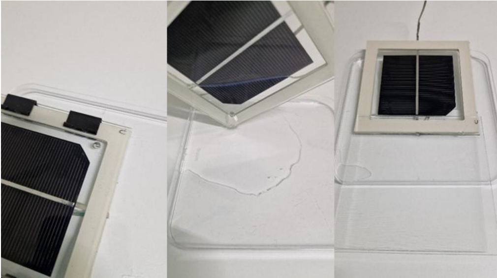
Figure 33. Draining of the encapsulant
