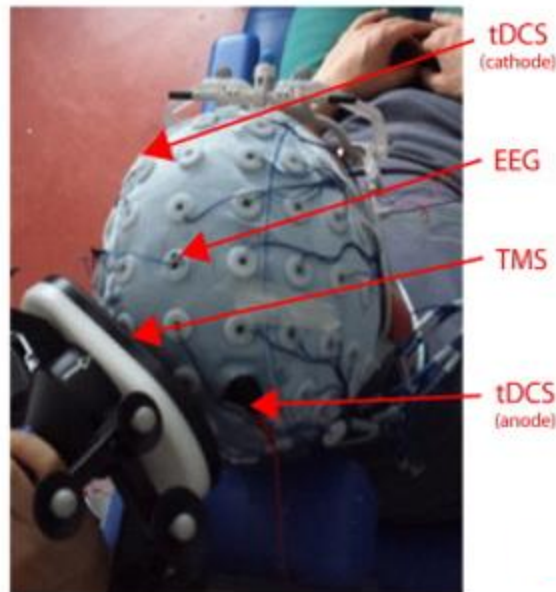
Figure 1-1: Image depicts the experimental arrangement employed to administer tDCS and TMS concurrently, with EEG recording conducted during tDCS. [12].
