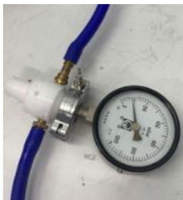
Figure. 15. Pressure gauges connect between pipes
