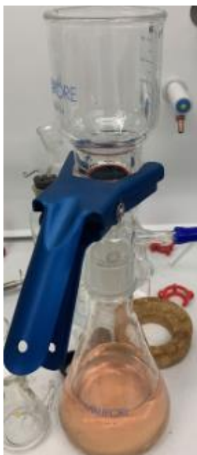
Figure. 14. Vacuum filtration equipment
