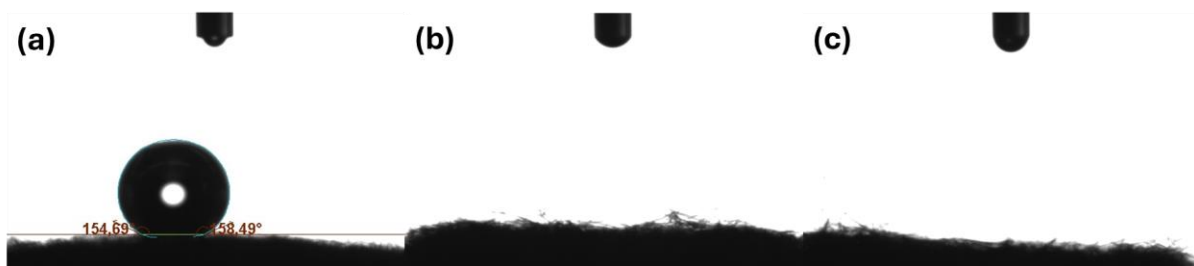
Figure 7. The contact angle images of (a) pristine (b) 5-dipped (c) 10-dipped graphene coated felts. Dropped liquid is distilled water.
